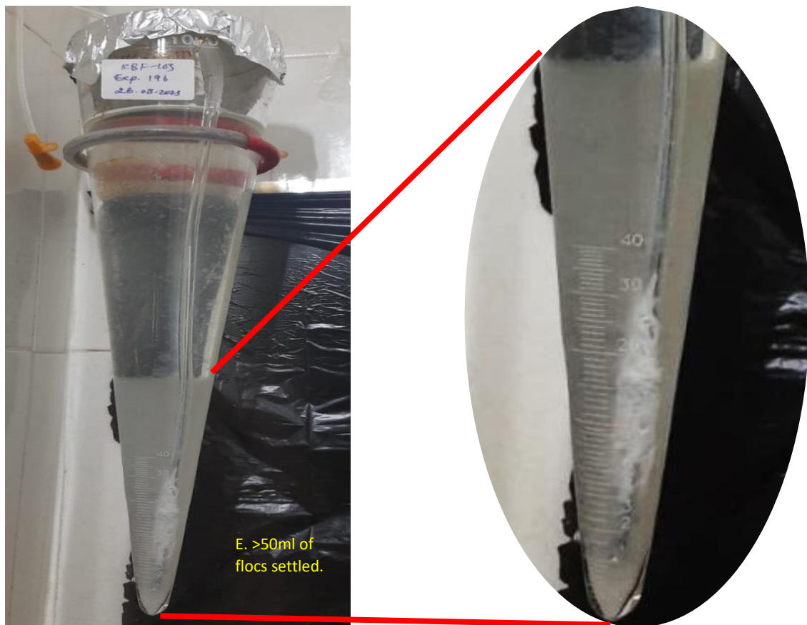
Figure 3. The biofloc generated by strain KBF-103 was examined using an Imhoff cone and checked under a microscope at various magnifications: a (4x), b (10x), c (40x), d (100x), and e. the settled KBF-103 flocs were found at the bottom of the cone.
