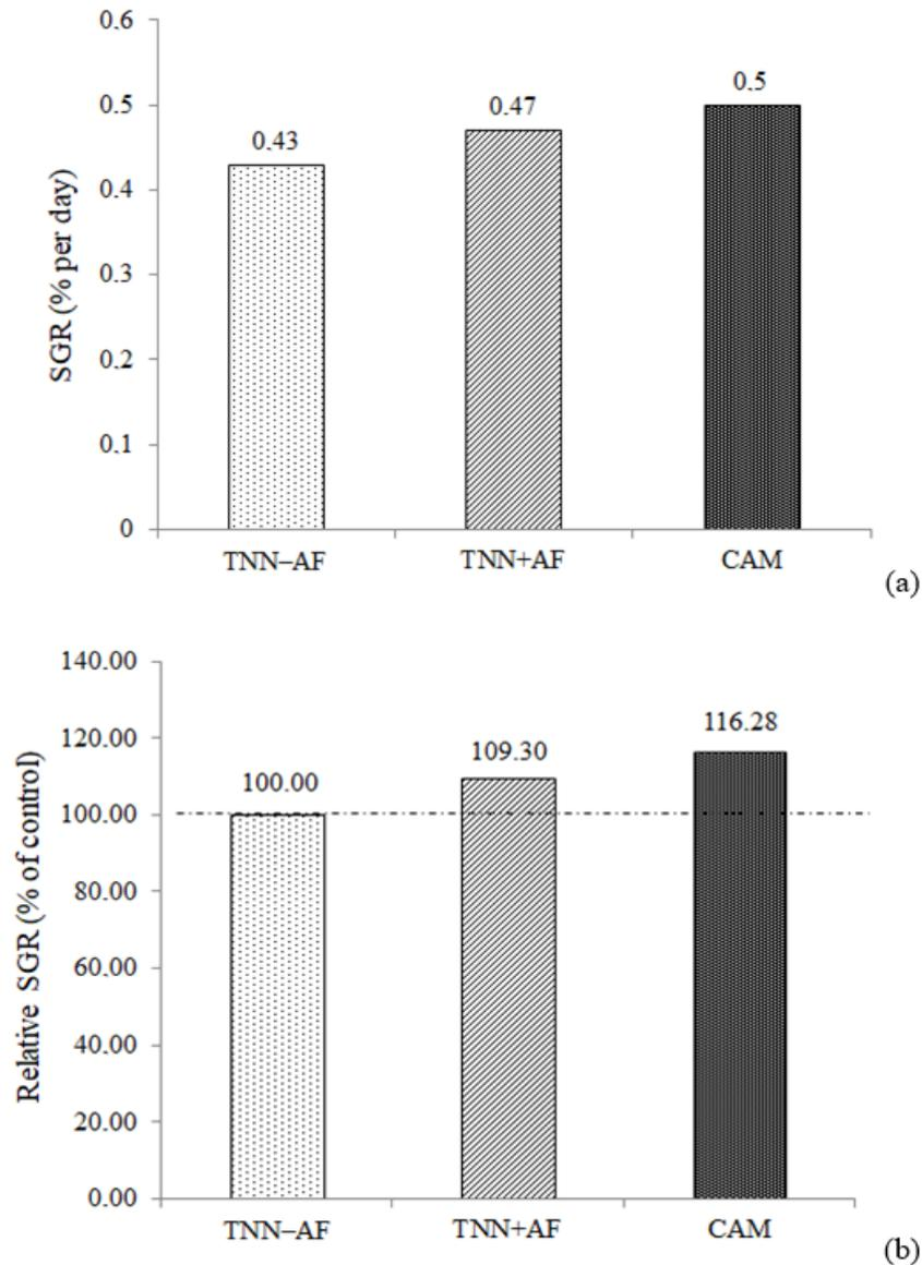
**Figure 2.** Specific growth rates of gilthead seabream in antifouling treated (TNN<sub>+AF</sub>) and copper alloy mesh (CAM) pens (a) and SGR relative to the control group with non-antifouling treated polymer net (TNN<sub>-AF</sub>) (b).
