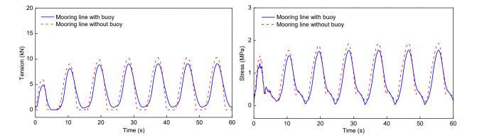
Figure 4. Mooring line tension and von Mises stress at point A under pure wave conditions with a height of 5 m and period of 9s.
