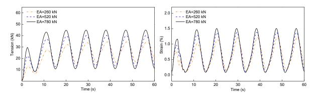
Figure 11. Mooring line tension and deformation of the floating collar with different axial stiffness values.
