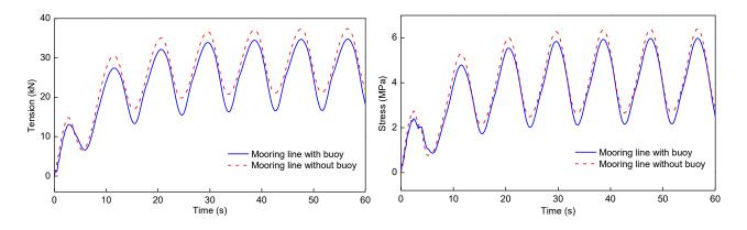
Figure 6. Mooring line tension and von Mises stress at point A under a wave height of 5 m, period of 9 s, and current velocity of 1.0
