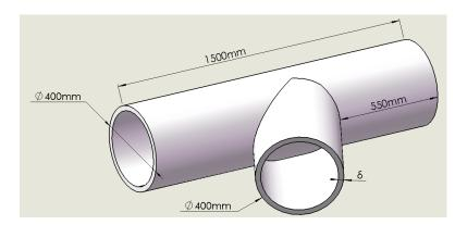
Figure 8. Component for connecting the floating pipes.
