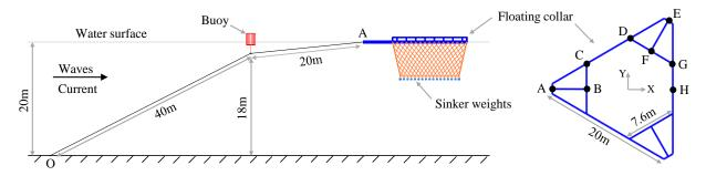
Figure 2. Schematic representation of the SPM cage system.
