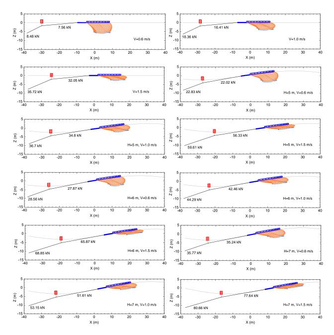
**Figure 7**. Deformation of the SPM cage system at the instant of maximum mooring line tension occurrence under waves combined with currents. The top line is the water surface.
