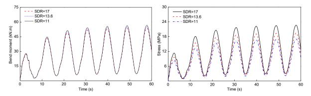
Figure 9. Bending moment and von Mises stress at point D attached to the connected component with various values for SDR.
