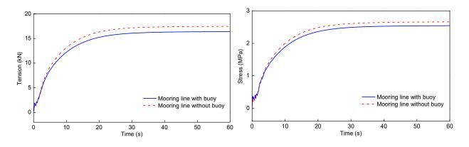
Figure 5. Mooring line tension and von Mises stress at point A under a current velocity of 1.0 m/s.
