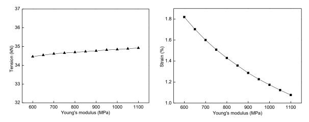
Figure 10. Mooring line tension and deformation of the floating collar with different values of Young's modulus.
